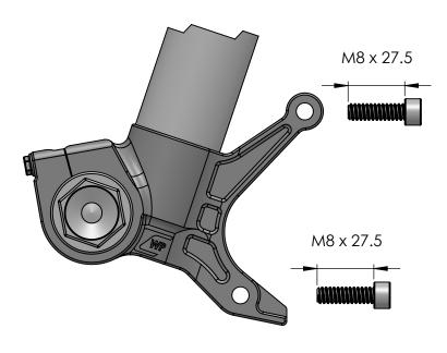
Use the included Moto-Master M8 x 27.5 mm bolts to mount the caliper adapter bracket.
